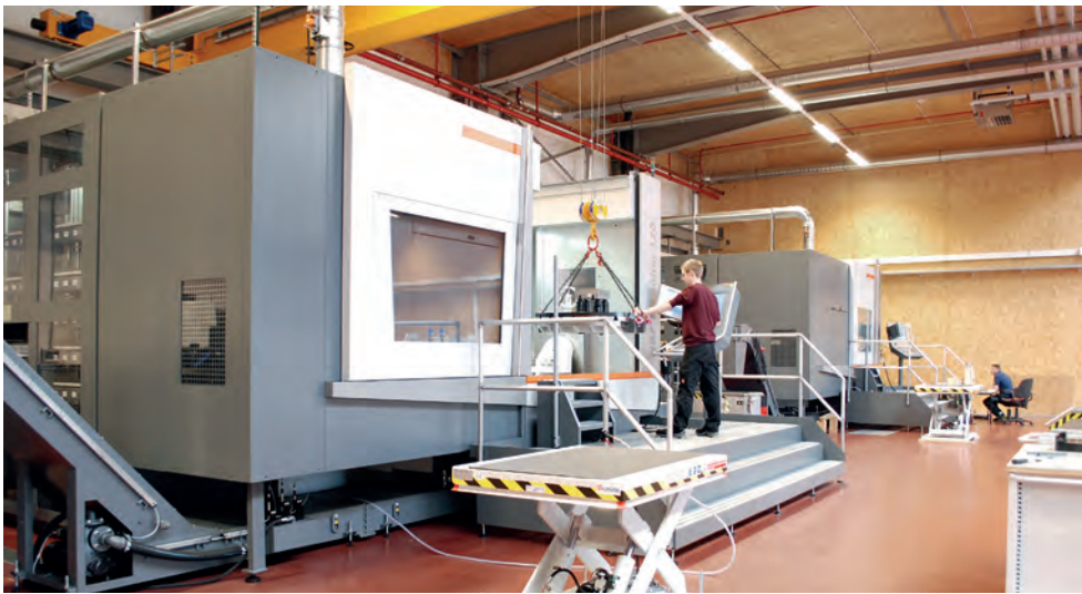
■ Horizontal milling machining centres (above) and portal grinding machine (right) for the production of mould plates
