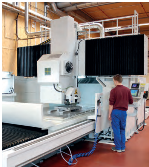
■ Horizontal milling machining centres (above) and portal grinding machine (right) for the production of mould plates
