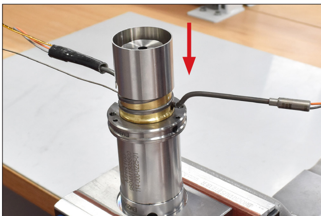
Picture 106: Installation of the new thermocouple, installation of the protective tube
